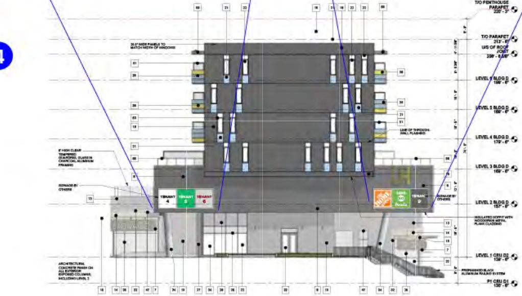
2 BUILDING D - SOUTH ELEVATION SCALE: 1/8" = 1'-0"
